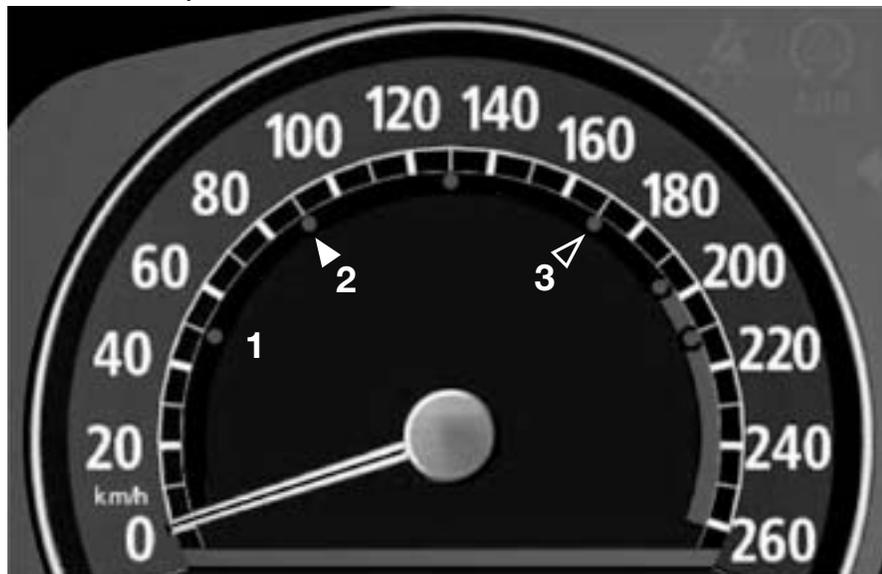
Briefly press/pull the lever to illuminate the cruise control mask in the speedometer. The memory will accept and store up to 6 preset speeds. When the cruise control is not active, the silhouette pointer indicates the last speed at which it was activated.
