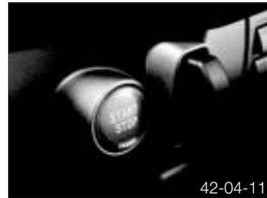
When starting to the engine, the CAS contains the data for the EWS code which is transferred to the ECM. The transmission of EWS data between the CAS and the ECM is over the data line D - EWS. Terminal R and terminal 15 is directed by the CAS for all electrical systems. The CAS also activates KL15 WUP (Wake UP) for control modules on the PT-CAN.
