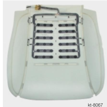
As of a weight of approx. 12 kg (26.4lbs.), the seat is recognized as occupied. The electronic evaluation units of the seat occupation mats are connected to the relevant satellites. (SSFA/SSBF=sensors for front seat, SSH=sensors for rear seat)
