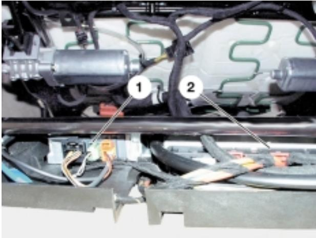
The satellites of the driver and passenger side are identical. The satellite is located below the seat frame between the seat rails. It is fitted with the seat module beneath a cover in a plastic tray.
