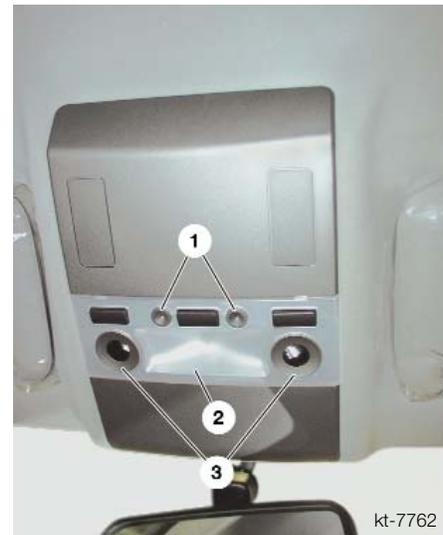
The ambient lighting LEDs are supplied power by the KL-58g circuit of the Light Module.
