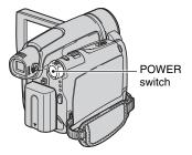
1 Slide the POWER switch repeatedly in the direction of the arrow to turn on the respective lamp.
