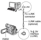
You can only use an i.LINK cable for this operation. You cannot use a USB cable.  For DCR-HC44E/HC46E/HC94E/ HC96E:
