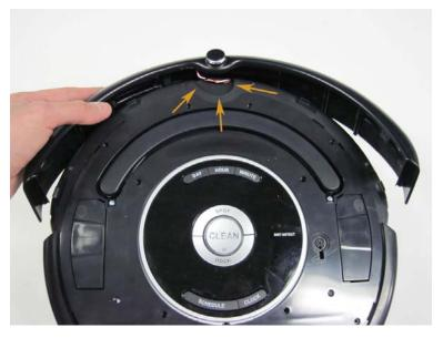
3.2.9 Place the bumper properly on the front of the unit, over the top cover.
