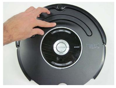
3.2.16 Do the same for the bottom half of the faceplate. Push down firmly on the bottom left and right corners of the faceplate until you hear/feel it click into place, or until the faceplate is flush with the top of the robot.
