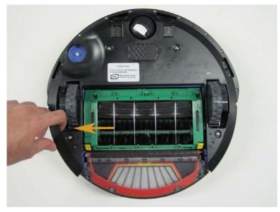
3.1.6 ...and remove the bottom cover from the robot.
