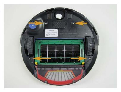
3.1.5 Once the cover is loose, using one of your fingers, hook the bottom cover near the openings for either drive wheel...
