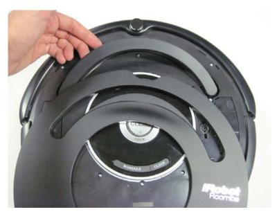
3.2.13 Push the curved tab underneath the handle, while slipping the front edge of the faceplate over the top of the handle.
