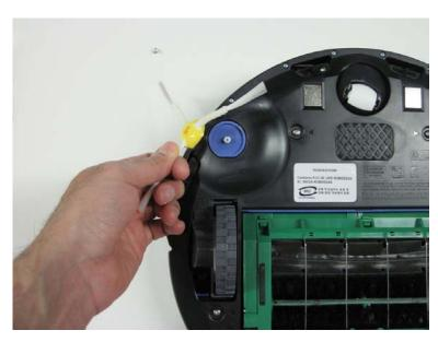
3.1.4 Loosen the four screws holding the bottom cover in place.
