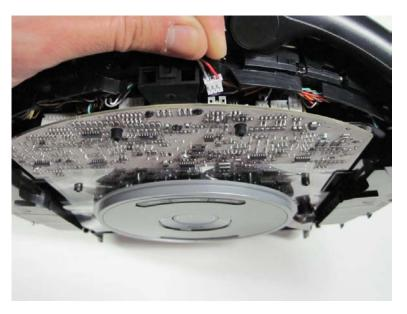
3.2.3 Due to the angle, the connector may be difficult to install all the way without bending backwards the socket on the motherboard. You may want to carefully use a flattipped screwdriver (or similar tool) to gently push the connector into place, all the while pushing slightly inwards toward the motherboard to keep the socket from bending.
