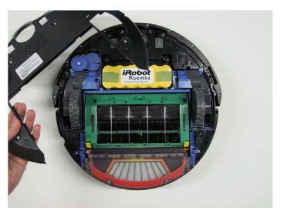
3.1.7 Now remove the battery, lifting it out of the robot using the pull tabs on each end of the battery.
