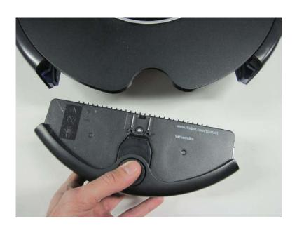
3.1.12 Remove the faceplate from the Roomba. Starting at the bottom where the dustbin goes, lift up the edge of the faceplate, and insert a long screwdriver (or similar tool) into the gap. Then, while holding the Roomba in place, lift the handle end of the screwdriver like a lever to un-clip the faceplate from the Roomba.
