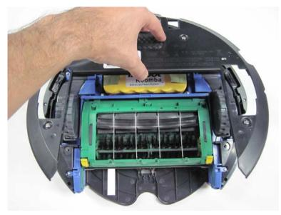
3.2.22 Tighten the bottom cover's four screws until the cover is no longer loose.
