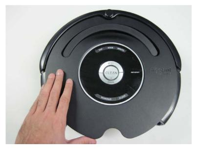
3.2.15 To fasten the front end in place, push down firmly on the top/front part of the faceplate until you feel/hear it click into place, or until the faceplate is flush with the top of the robot.
