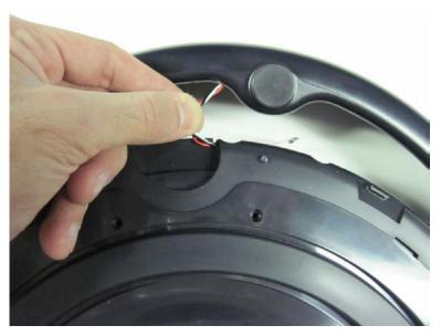
3.2.8 Push the top cover down into place on the frame. Position the wiring for the bumper so that any slack in the wires curls around, following the shape of the groove on the front of the top cover, as shown by the orange arrows.
