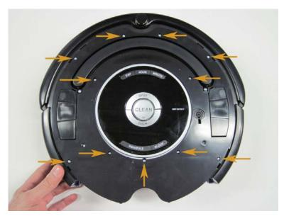
3.1.14 Loosen the top cover from the robot by lifting the edge of the cover up, while pushing down on the main frame with your thumb, as pictured.
