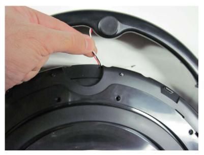
3.2.7 Push the wires into the slot provided on the front end of the top cover. The opening for the slot is small, so you may have to push in one wire at a time.
