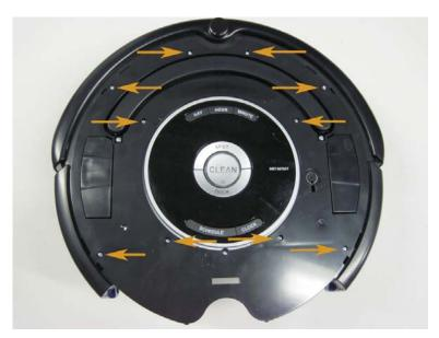
3.2.12 To install the face plate, first lift the front handle.
