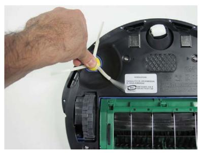
3.2.24 Only once the side brush has been clicked into place properly should you insert the screw into the center of the brush.
