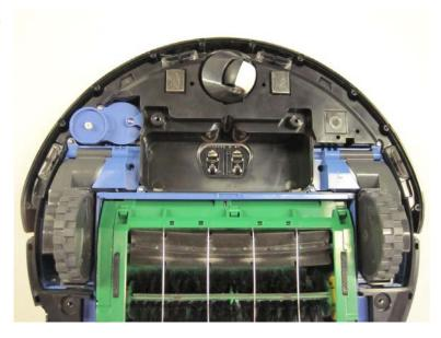
3.2.18 Place the front bumper's trim piece down on the bumper's underside, lining up the screws with the bottom of the front bumper.
