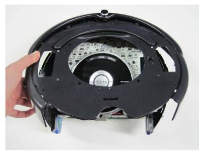
3.1.17 Unhook and remove the bumper wire from the top cover to remove completely the top cover from the robot.
