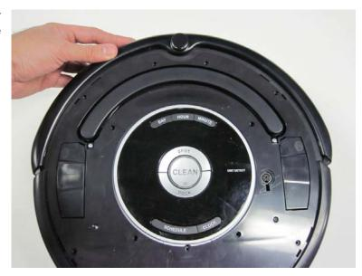
3.2.10 Insert the screw for the top cover, as shown by the orange arrow. It is the only screw of its size (smaller than all the others) that was removed from the top cover.
