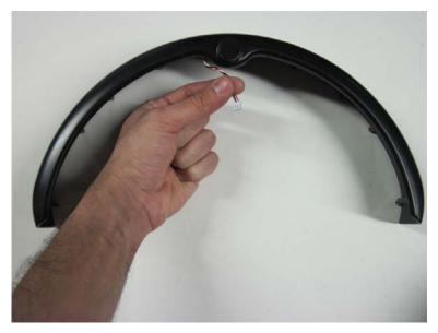
3.2.2 Reinsert the bumper wire connector into its socket.
