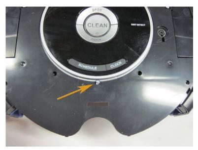
3.2.11 Insert the remaining screws for the top frame cover, as shown by the orange arrows.
