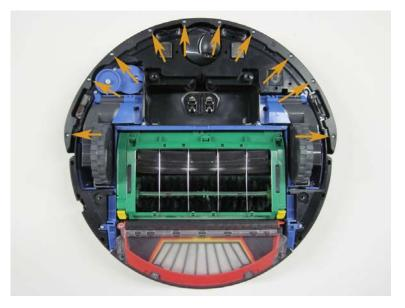
3.1.9 With the screws loose, now remove the bumper's bottom trim piece from the robot.
