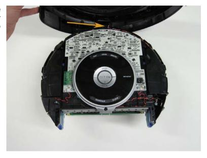
3.1.18 Once the top cover has been removed, the bumper wire remains to be removed.
